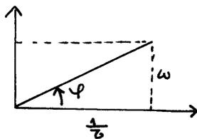
$$\begin{aligned} \underline{R} &= \frac{v_{x0}}{\frac{1}{\tau} \sqrt{1 + \omega^2\tau^2} \exp -j\varphi} \left(1 - e^{-t/\tau} e^{i\omega t}\right) \\ &= \frac{\tau v_{x0}}{\sqrt{1 + \omega^2\tau^2}} \left(\exp j\varphi - e^{-t/\tau} e^{i(\omega t + \varphi)}\right) \end{aligned}$$
